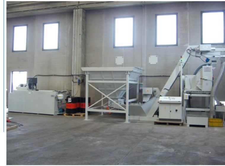
Automatic spinning plant with 6m3 pre-storage hopper
