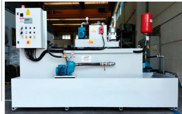
Oil filtration unit with automatic topping up
