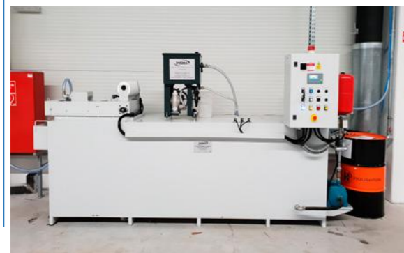
Centralized unit equipped with paper filter, tramp oil skimmer, dosing unit and automatic topping up
