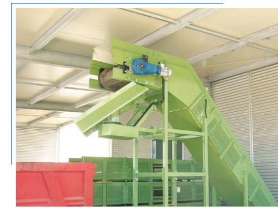
Detail of the discharge into container
