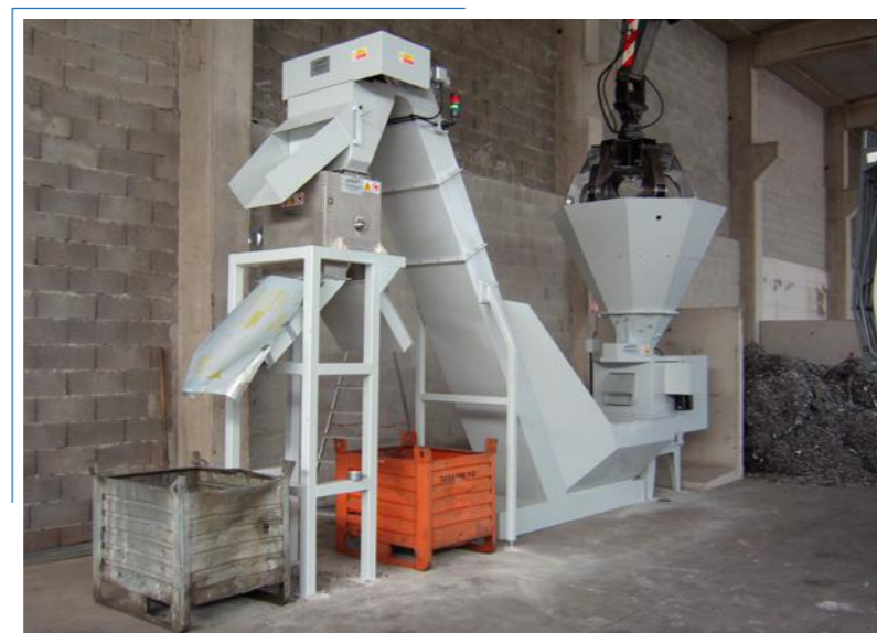
Automatic crushing system equipped with magnetic separator
