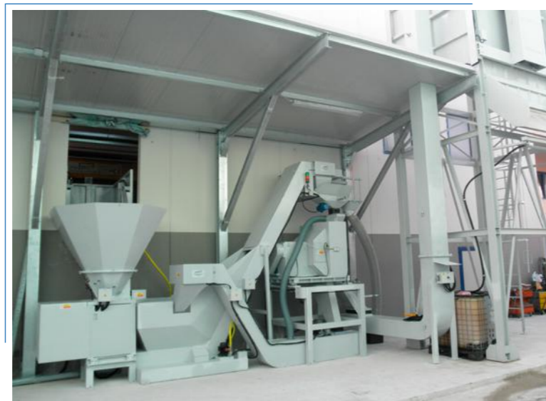
Swarf crushing and spinning plant with silos
