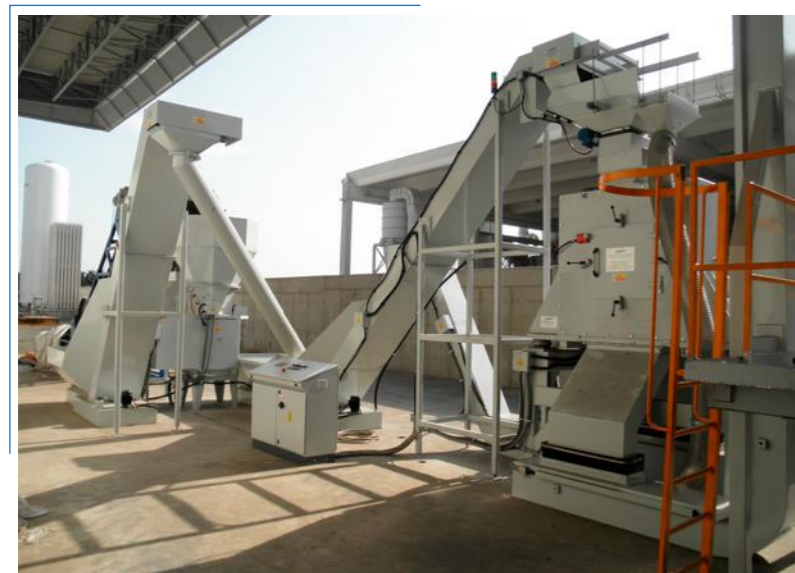
Crushing and spinning system. Capacity: 3 ton/h for aluminium swarf
