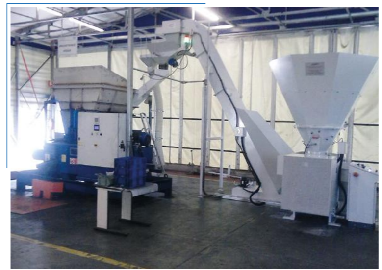
Automatic crushing and briquetting system
