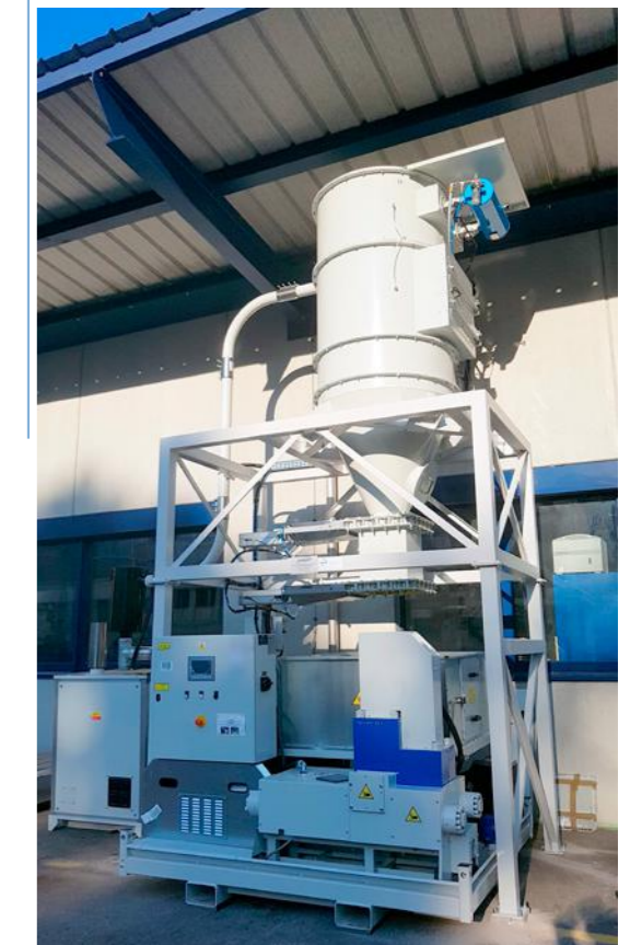
Vacuum plant feeding a briquetting machine
