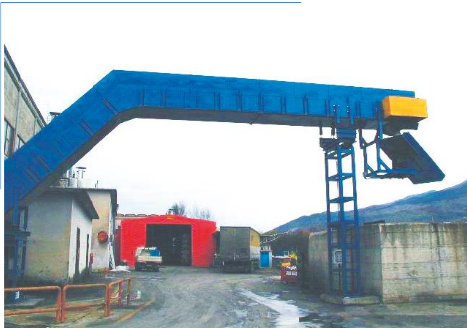
Heavy conveyor for scraps discharge
