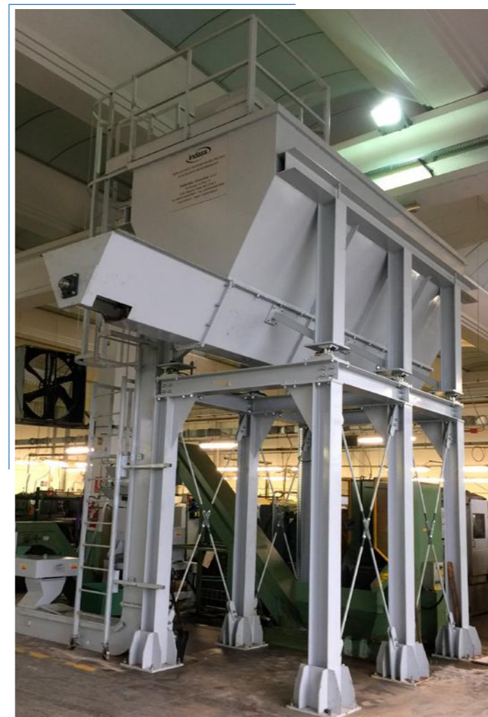
Horizontal silos equipped with load cells
