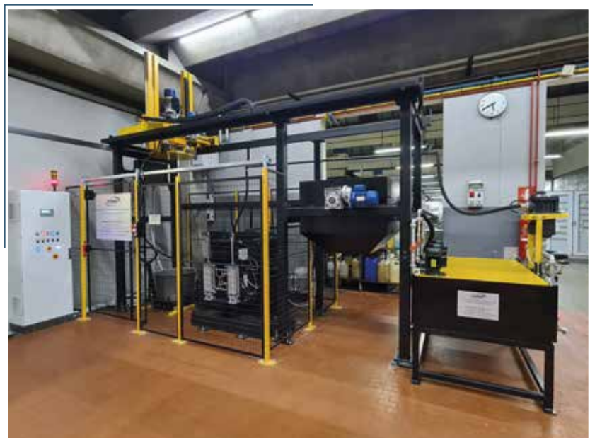
Plant with single discharge for multiple materials
