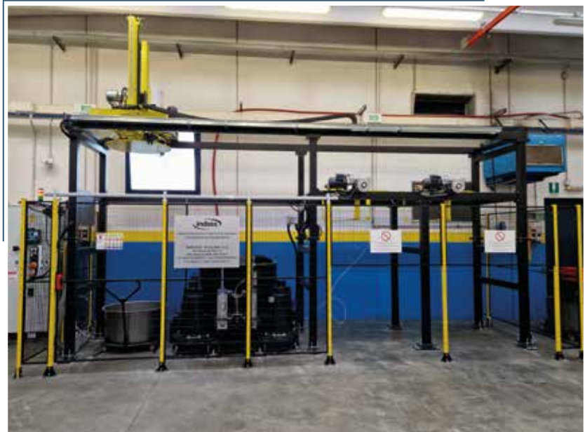
Plant with double discharge stations for multiple materials
