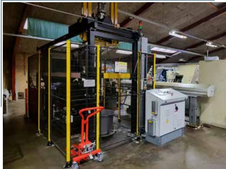
Plant with single discharge for multiple materials, with baskets access on the side
