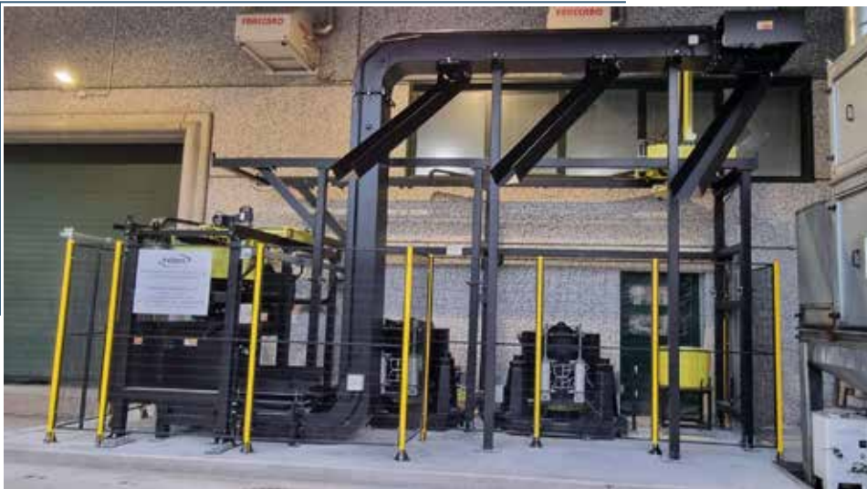
Plant with double centrifuge and double discharge station
